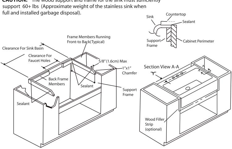
There should be a hole cut in the front of the cabinet face to accommodate the apron front as well. Measure sink apron and cabinet opening to make sure apron will fit into cabinet opening. If necessary, sand opening or add wood filler strips. Apron should rest against the cabinet face. This sinks apron can protrude 2 - 2 1/4" away from the cabinet wall, NOTE you MUST measure to accommodate this variance to determine actual hole depth for sink as well.
